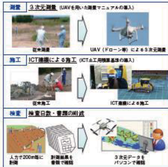
図表1-3-3 i-Constructionの推進 (ICT土工の流れ)
